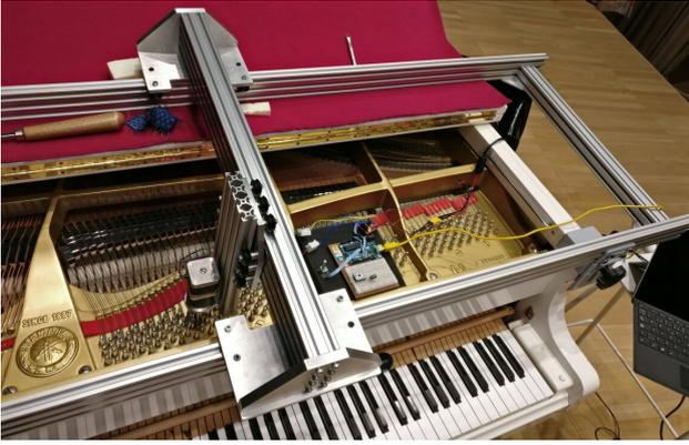
Figure 1. Proposed piano tuning system with the Arduino processor near the midpoint of the picture and the stepper motor on its left-hand side, attached to the topmost aluminum bar.
