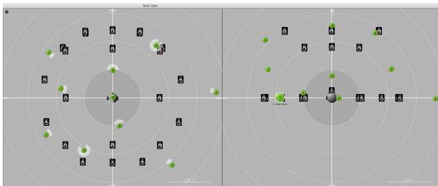
Figure 1. 10 sources distributed over the Sound Spatialization setup in the LIATe shown in the Max object spat5.oper .
