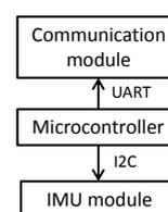
Figure 2. Block diagram of the remote control hardware.
